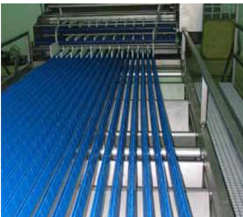
Fig. 1.2.3.i. Here we can see how the adjusting bars with the adjusting pins have been installed, grading channels getting installed and grading chains installed.
