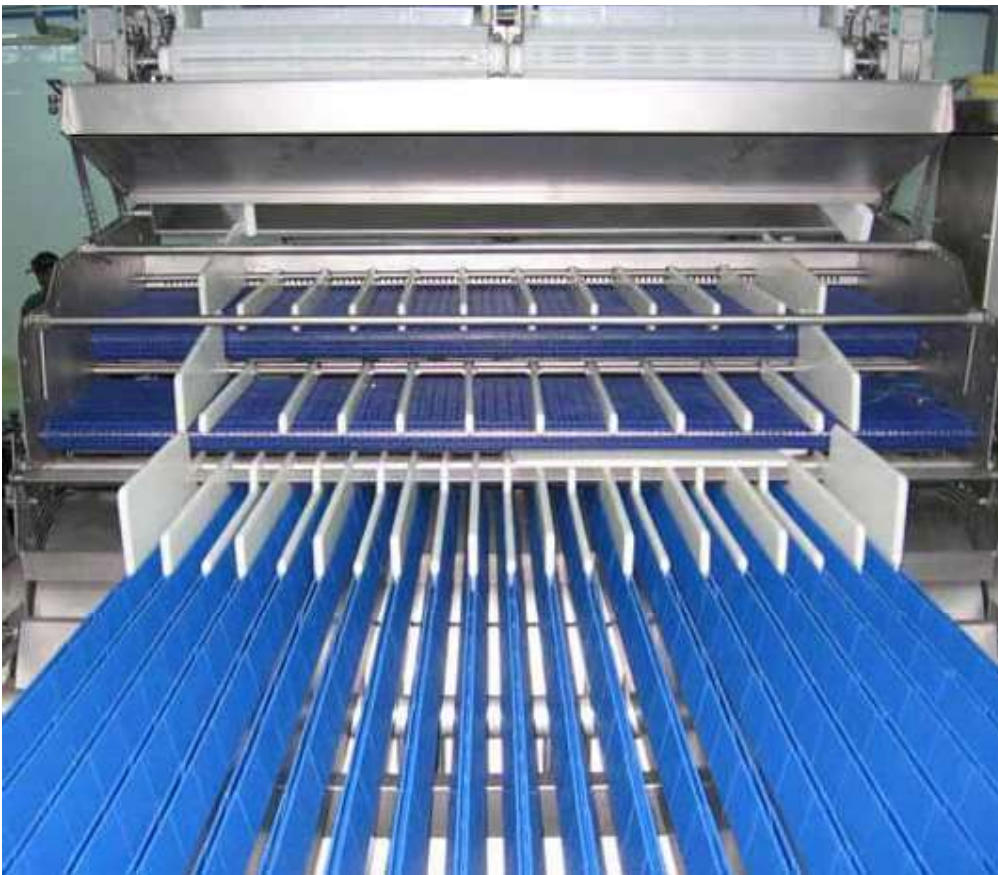
Fig. 1.2.2.g. Front-view of Style feeding system. Adjustable plates on top of conveyors.
