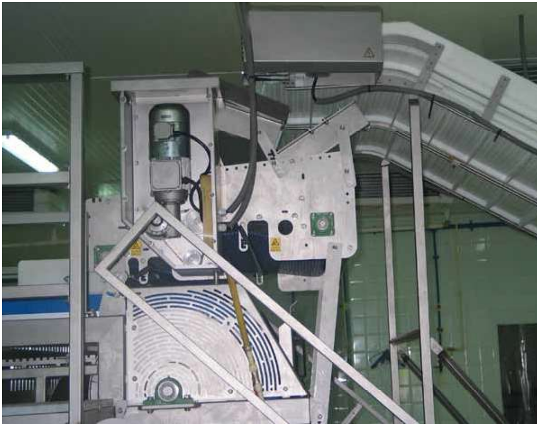
Fig. 1.2.2.i. Side-view of Style feeding system showing the motor and gear box.
