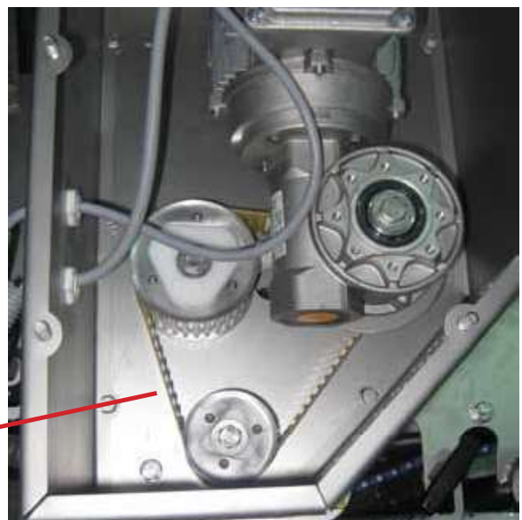
Fig. 1.2.2.k. Style feeding system. Motor and gear box.
