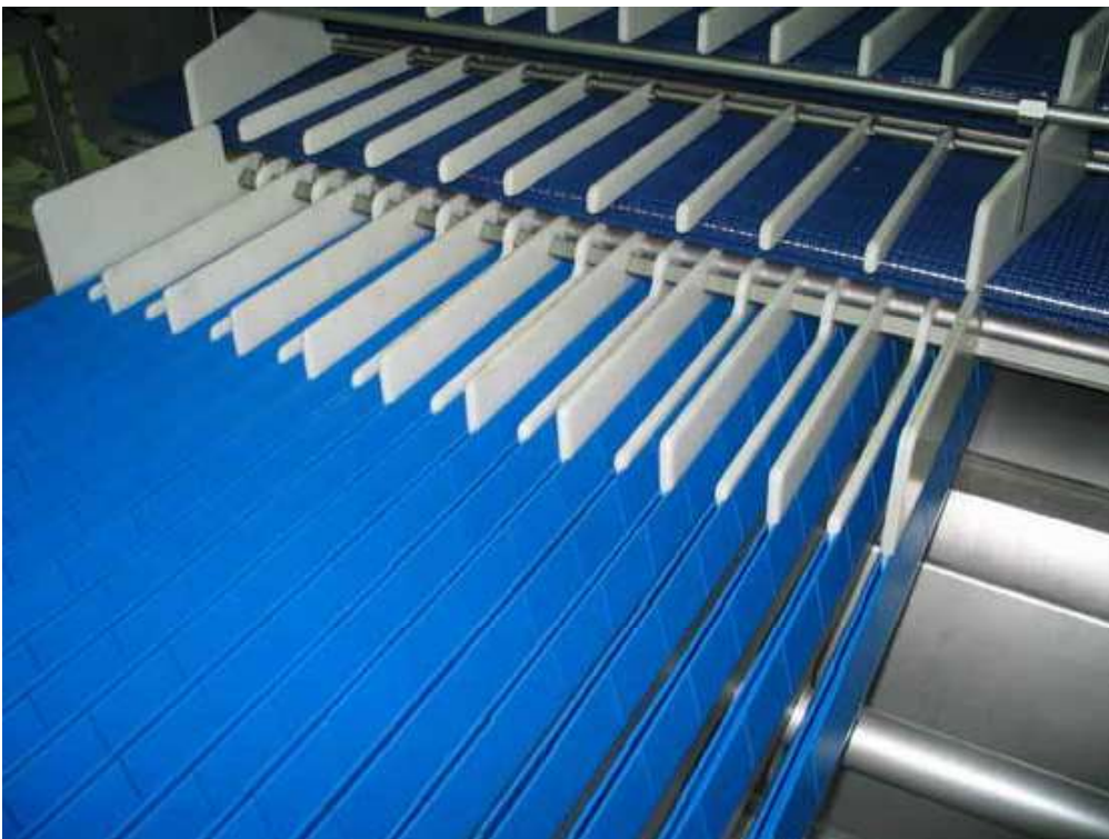
Fig. 1.2.2.h. Front-view of Style feeding system and grading channels on top of grader.
