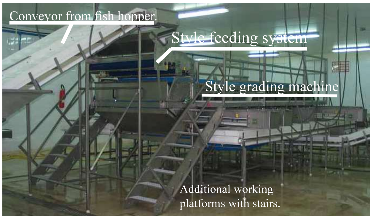
Fig. 1.2.2.a. Over all view of Style grading machine with feeding system and conveyor from hopper.
