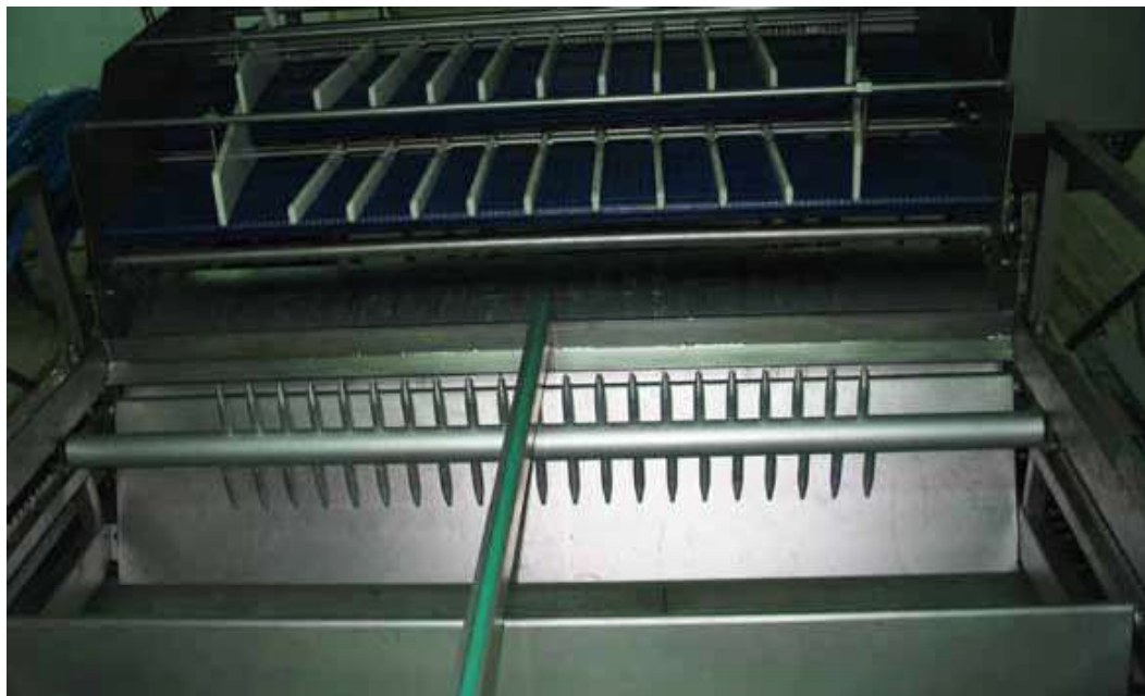
Fig. 1.2.3.f. Here we see how the first grading channel is then installed on top of the aluminium pins in the adjusting bars. Begin in the middle and end out at both sides until all the channels have been installed. No tool needed for this.
