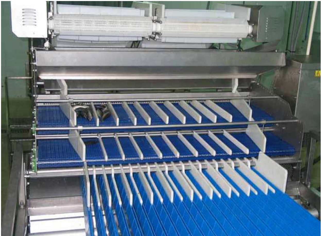
Fig. 1.2.2.e. Front-view of Style feeding system. Adjustable plates on top of conveyors.
