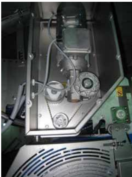
Fig. 1.2.2.j. Style feeding system. Motor and gear box.
