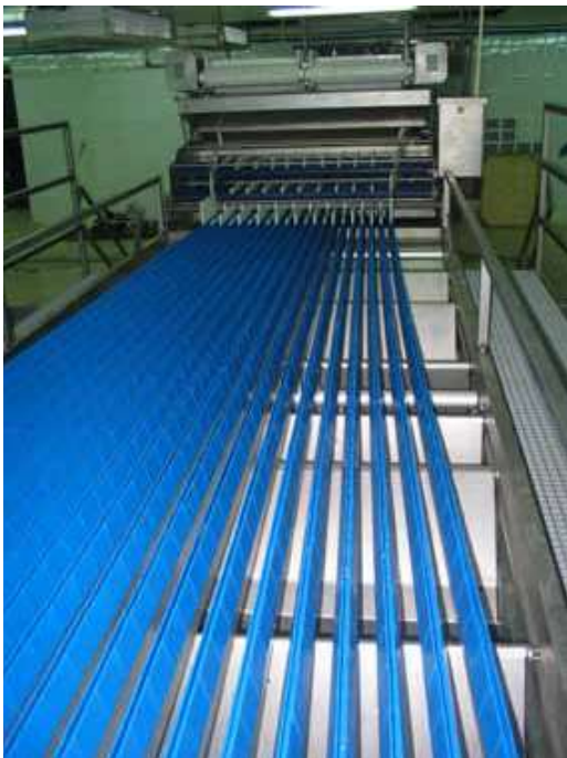
Fig. 1.2.2.f. Front-view of Style feeding system and grading channels on top of grader.
