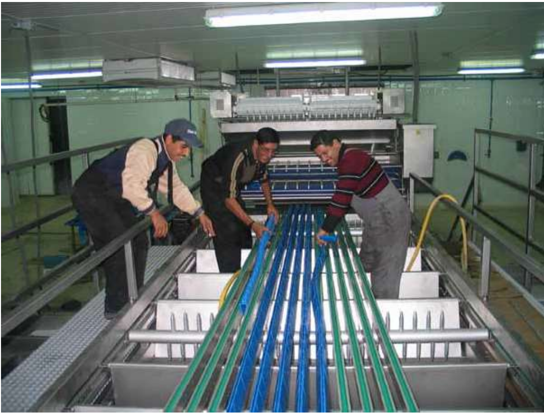
Fig. 1.2.3.g. Here we can see how the adjusting bars with the adjusting pins have been installed, grading channels getting installed and grading chains installed.
