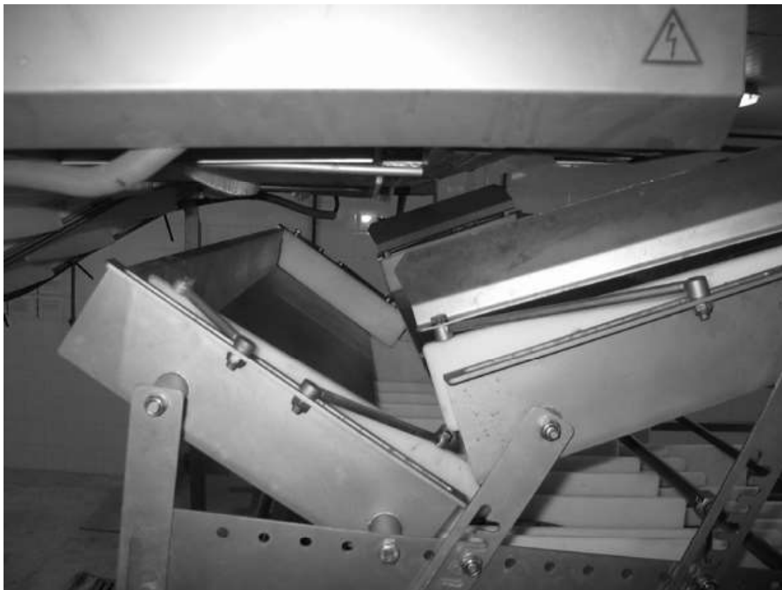
Fig. 1.2.2.d. Side-view of Style feeding system. Adjustable plates on top of feeding system
